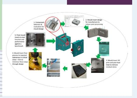
Injection Mould Tooling, Efficiency Enhancement Through Design Optimisation and Advanced Post-Processing Methods for Metal 3D-Printed Tooling
